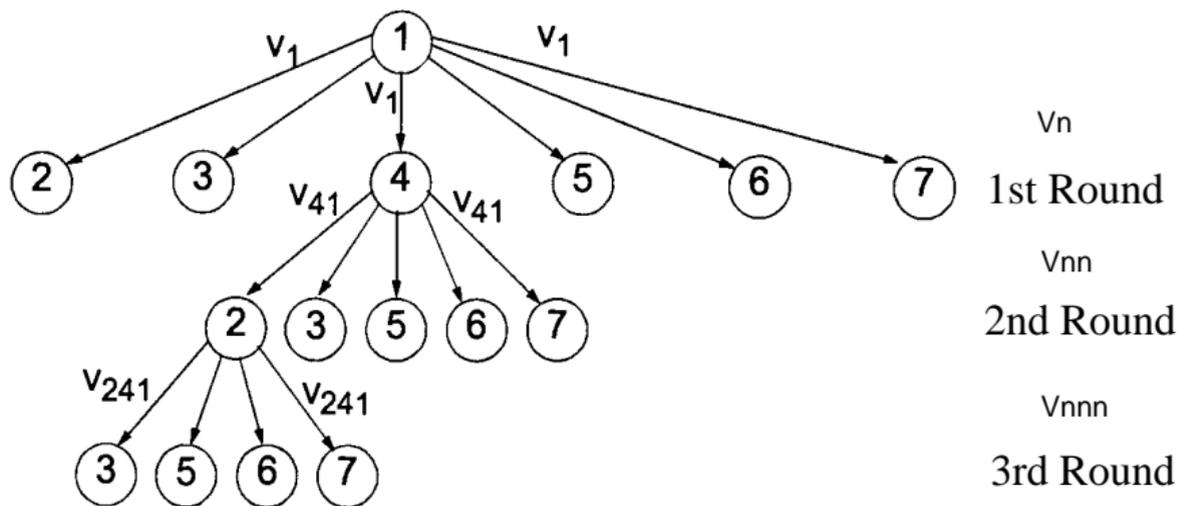
Unit 2 uses  $v'_1 = \text{majority}\{v_1, v'_{31}, v'_{41}, v'_{51}, v'_{61}, v'_{71}\}$
