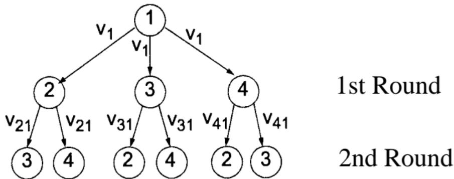
Unit 2 uses  $v'_1 = \text{majority}\{v_1, v_{31}, v_{41}\}$
