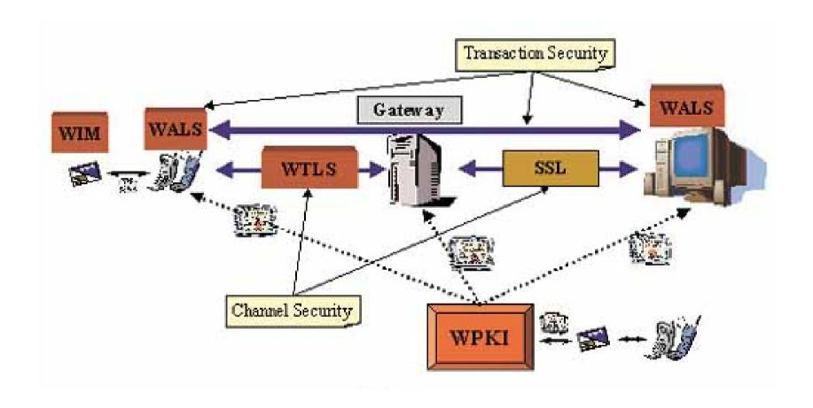
WALS contains Digital signature and encryption at application layer. But standard method doesn't exits yet.
