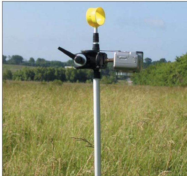
Figure 1. A photographic technique for measuring percent ground cover of vegetation used in nine fields in northwest Arkansas during 2003. A Kodak DC4800 Zoom Digital Camera mounted on a telescoping pole at a height of 1.5 m was used to photograph an approximately 2 m 2 area centered on the nest.
